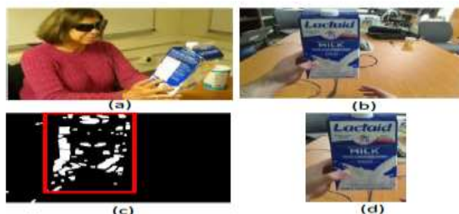
Fig. 1. Localizing the image region of the hand-held object of interest. (a) Capturing images by a camera mounted on a pair of sunglasses; (b) An example of a captured image; (c) detected moving areas in the image while the user shaking the object (region inside the bounding box); (d) Detected region of the hand-held object for further processing of text recognition.
