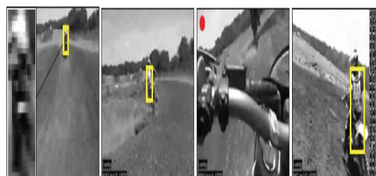
Fig. 7 Given a single bounding box defining the object location and extent in the initial frame (LEFT), our system tracks, learns, and detects the object in real time. The red dot indicates that the object is not visible.
