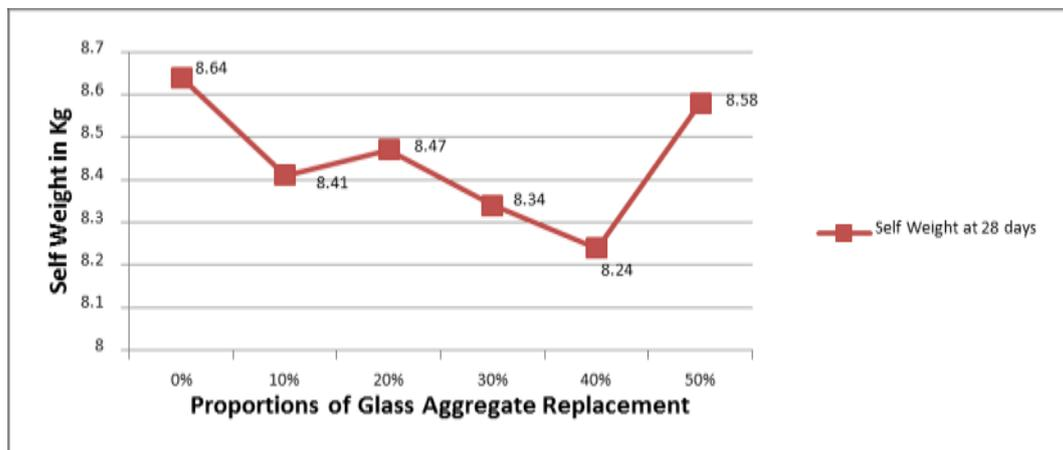
Fig.2: Graph Indicating Comparison between Self Weights of Conventional Concrete with Modified Concrete.
