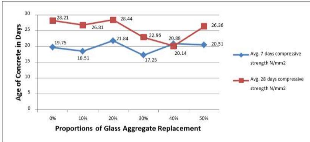
Fig.1: Graph Indicating Comparison between Compressive Strengths of Conventional Concrete with Modified Concrete.
