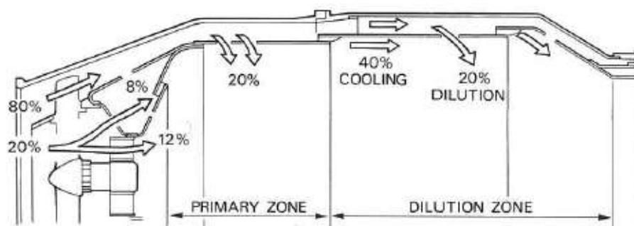
Fig- 2 Airflow Distribution along the chamber
