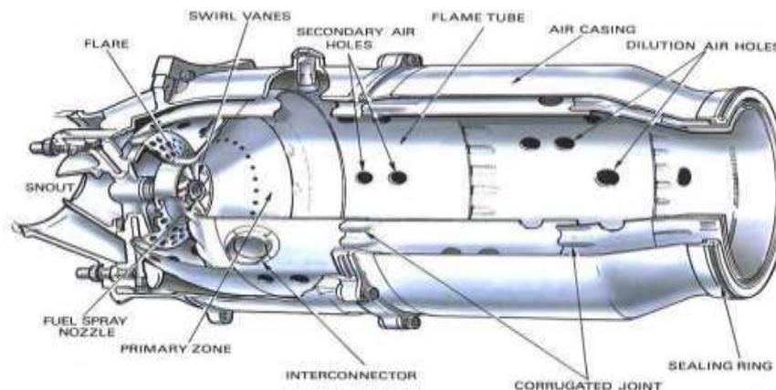
Fig -1 Combustion Chamber
