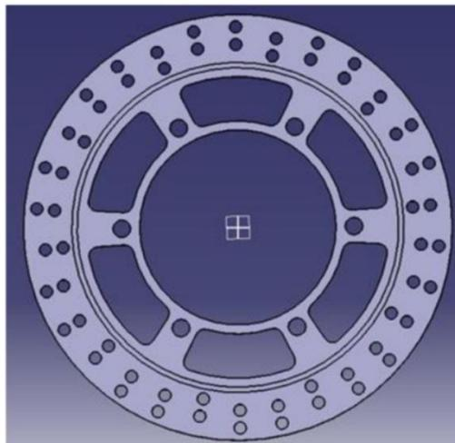
Fig. 2. 3D Modeling of shape 4 of disc brake rotor
