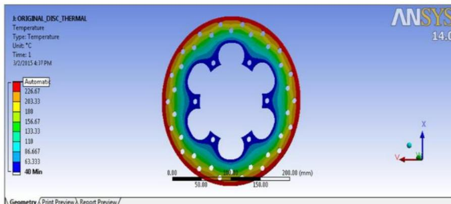
Fig.4. Steady state Temperature of original disc brake rotor
