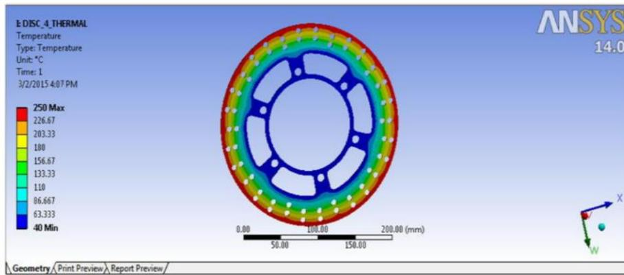
Fig.5. Steady state Temperature of modified shape 4 disc brake rotor
