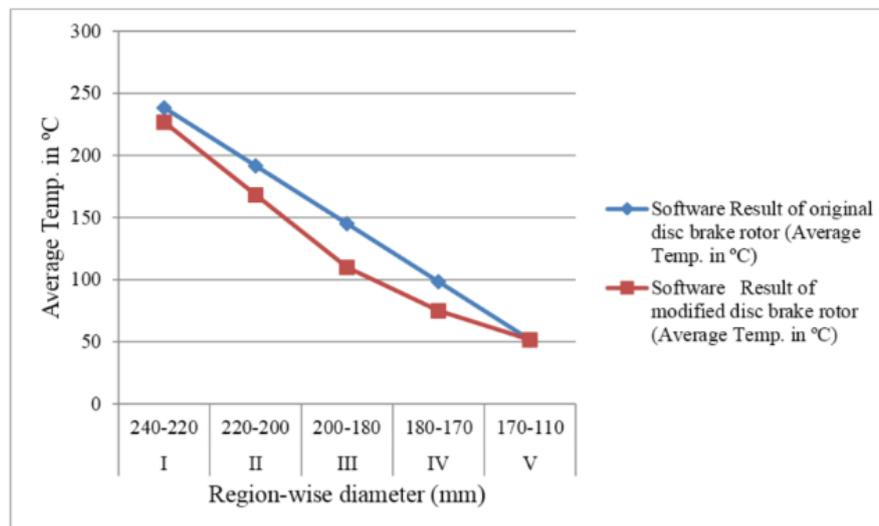
From above graph on the basis of software results it is clearly understand that average temperature occurs in modified shape 4 disc brake rotor is minimum as compared to original disc brake rotor
