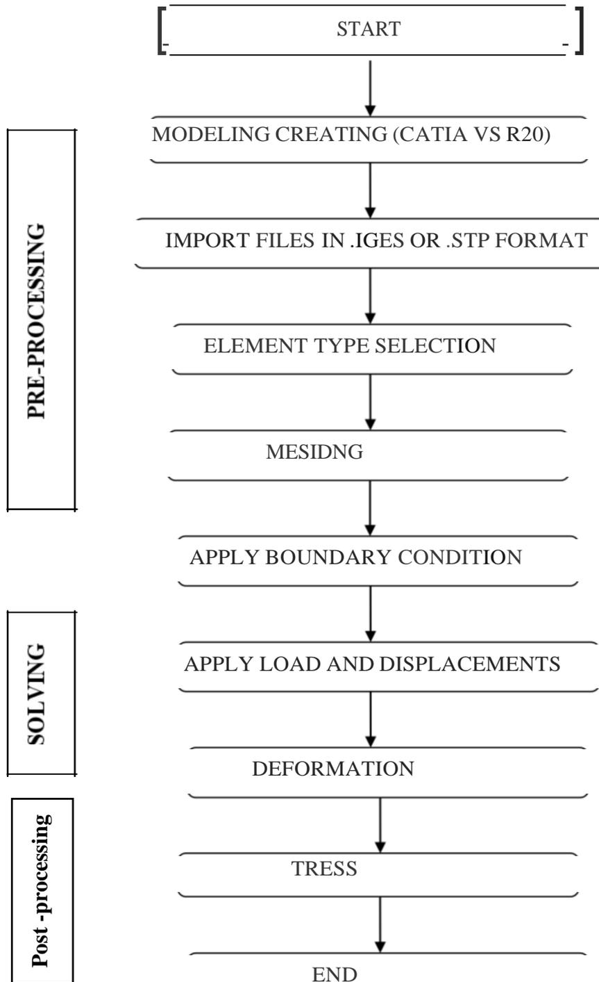
Fig 3: Flow Chart of Finite Element Method (Structural Analysis)
